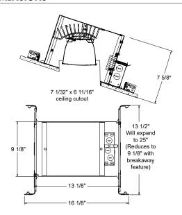
Mounting Frame 22-gauge die-formed galvanized steel mounting frame • Rough-in section (junction box, mounting frame, housing and bar hangers) fully assembled for ease of installation.
