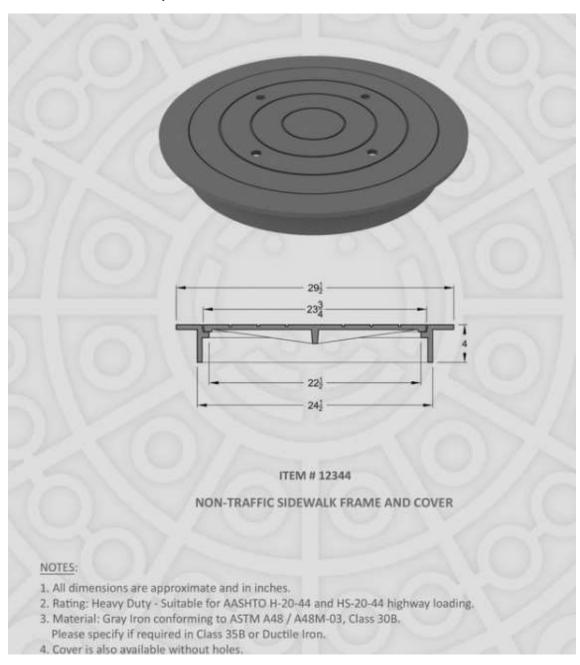
\* Std. depths 1½", 2", 2½" & 3" Matl. to be grey cast Iron ASTM A 48, Class 35B. Tolerance on non-machined surfaces to be |0.06", see general note 6
