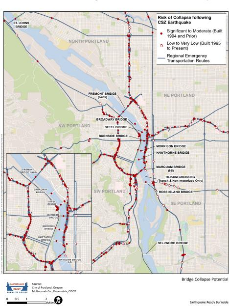
Figure S-3. Potential for Bridge and Road Structure Collapse/Failure
