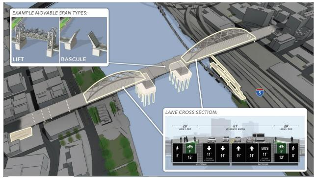
Note: The Draft EIS Long-span Alternative included multiple bridge types for both the east and west approaches. This figure shows only the tied-arch option.
