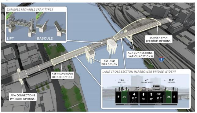
Notes: The Refined Long-span Alternative evaluated in this SDEIS includes both cable-stayed and tied arch options for the east span. This figure shows only the tied arch option. The Draft EIS studied, and SDEIS further studies, a bascule option and vertical lift option for the center movable span. The inset shows both options but the main figure shows the bascule option. This figure also shows just one of the lane configuration options considered in the SDEIS.
