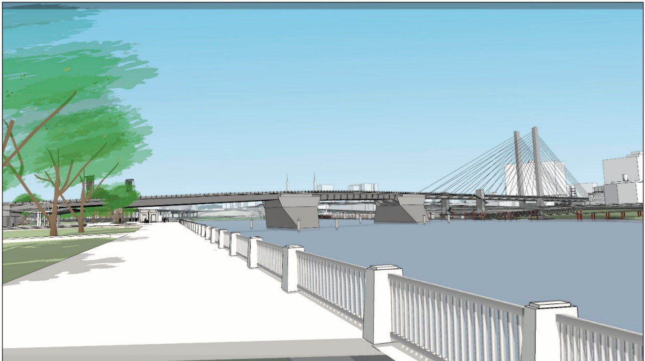
Figure 46: Span Combination 3 (girder west approach, bascule central span, cable supported east approach), artist's rendering, view looking north (Fat Pencil Studio, 2021).
