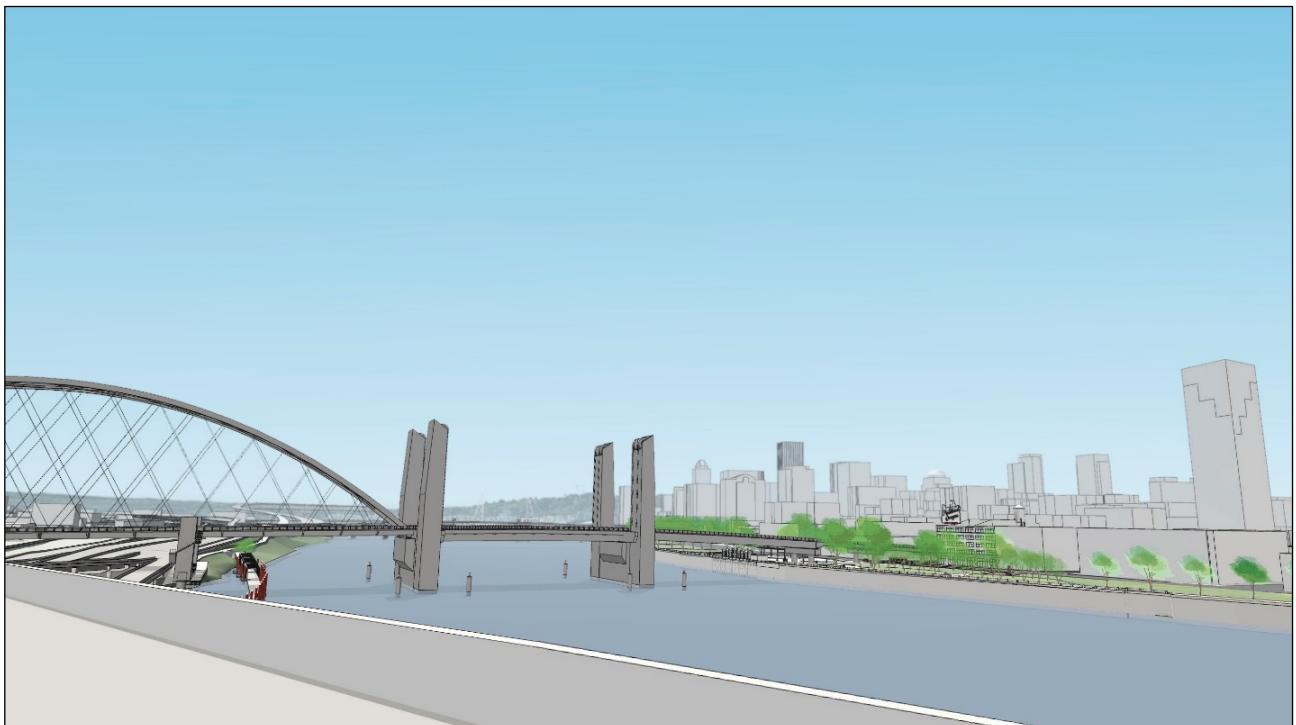
Figure 40: Span Combination 2 (girder west approach, vertical lift central span, tied arch east approach), artist's rendering, view looking south (Fat Pencil Studio, 2021).
