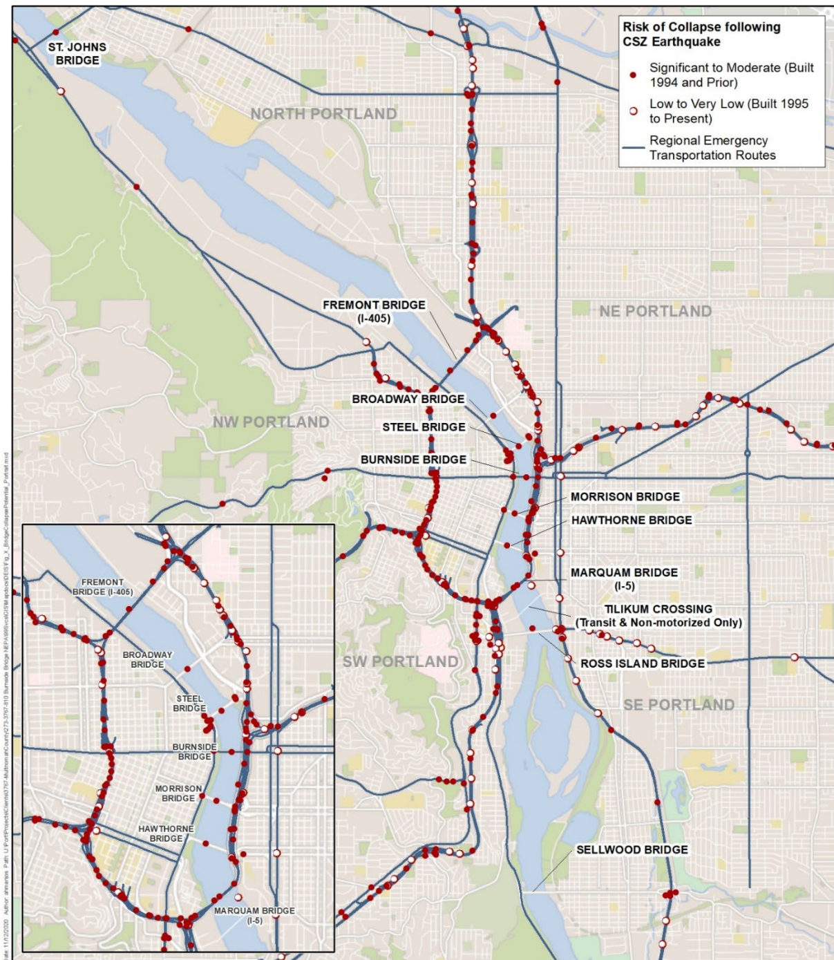
Figure 3-1. Bridge Collapse Potential
