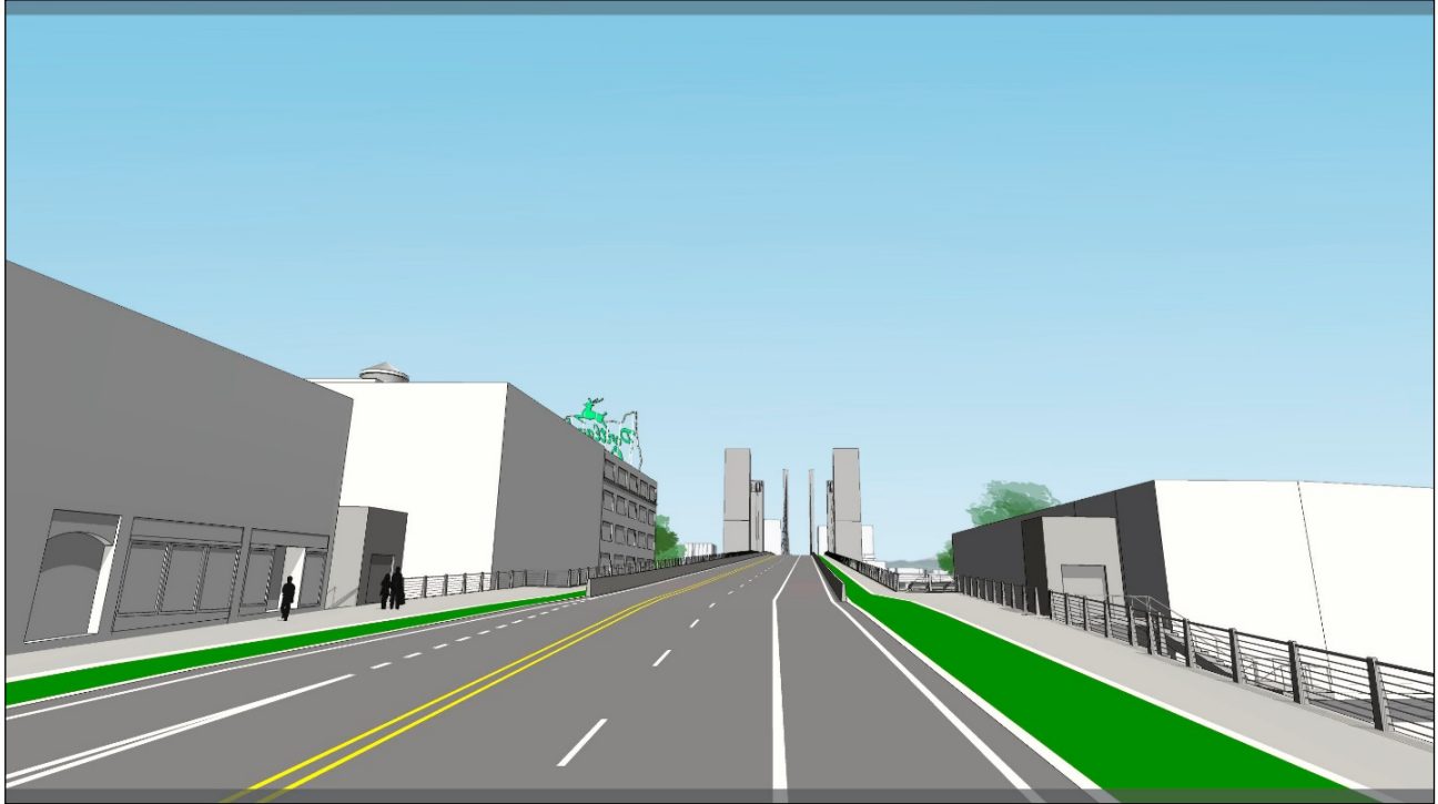
Figure 67: Span Combination 4 (girder west approach, vertical lift central span, cable supported east approach), artist's rendering, view looking east (Fat Pencil Studio, 2021).
