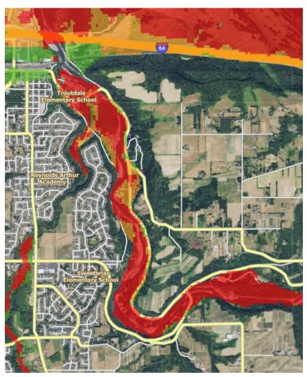
Figure 168 - Map showing soil liquefaction risks around Sandy River bridges. Red indicates high soil iquefaction risk, orange is moderate risk, and green are lower risk. Map from DOGAMI HazVu site.
