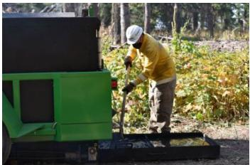
Figure 45 - The US Forest Service using a smokeless air curtain burner to turn debris into biochar. A large burner can process a ton of debris every hour.
