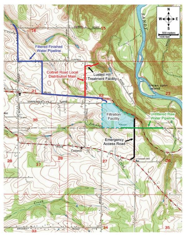
Figure 1. Location of the Bull Run Filtration Facility parcel (blue shading), RW pipeline (green line), FW pipeline (dark blue line), the Cottrell Road local distribution main (red line) to the existing Lusted Hill Treatment Facility, and the proposed emergency access road (black line) (USGS Sandy, Oregon 7.5' quadrangle, 1961, photorevised 1985).
