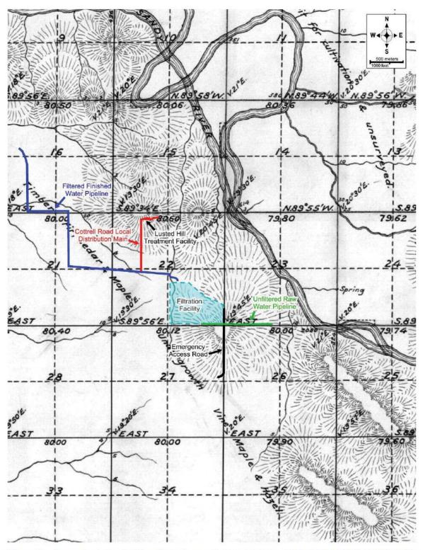
Figure 6. Excerpt of the GLO cadastral survey plat for T1S, R4E (GLO 1855) showing the proposed location of the Bull Run Facility parcel (blue shading), RW pipeline (green line), FW pipeline (dark blue line), the Cottrell Road local distribution main (red line) to the existing Lusted Hill Treatment Facility, and the proposed emergency access road (black line).
