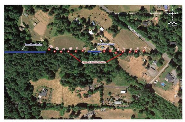
Figure 4. Location of shovel probes along the open-cut trench pipeline sections and the trenchless pipeline sections of the proposed RW pipeline between SE Lusted Road and the Facility (adapted from a July 24, 2021, Google Earth aerial photograph).
