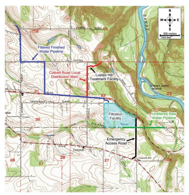
Figure 1. Location of the Bull Run Filtration Facility parcel (blue shading), RW pipeline (green line), FW pipeline (blue line), the Cottrell Road local distribution main (red line) to the existing Lusted Hill Treatment Facility, and the proposed emergency access road (black line) (USGS Sandy, Oregon 7.5' quadrangle, 1961, photorevised 1985).
