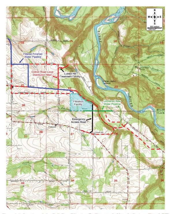
Figure A-1. Location of the Bull Run Filtration Facility parcel (blue shading), unfiltered RW pipeline (green line), filtered FW pipeline (dark blue line), the Cottrell Road local distribution main (red line) to the existing Lusted Hill Treatment Facility, the proposed emergency access road (black line), and unselected alternatives (dashed red lines) (USGS Sandy, Oregon 7.5' quadrangle, 1961, photorevised 1985).
