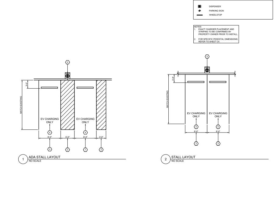
ACCESSIBILITY KEYNOTES (#) 1 VAN ACCESSIBLE STALL. 2 ACCESS AISLE. 3 STANDARD STALL. 4 SURFACE MARKING TO READ "EV CHARGING ONLY". 5 ACCESSIBLE IDENTIFICATION SIGN(S).
