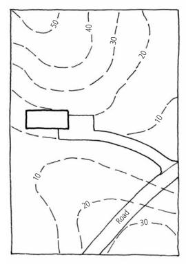
The structure and access drive are aligned with the slope to avoid excessive grading.
