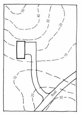
The structure and access drive are perpendicular to the contour lines, requiring more grading and more visible cuts and fills.
