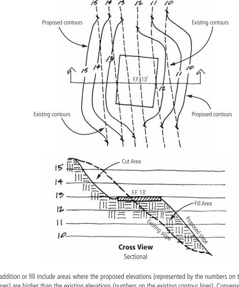
Areas of addition or fill include areas where the proposed elevations (represented by the numbers on the proposed contour lines) are higher than the existing elevations (numbers on the existing contour lines). Conversely, areas of removal or cut include areas where proposed elevations are lower than the elevation of the existing contour lines. Note: This figure exaggerates vertical slopes for illustration purposes.
