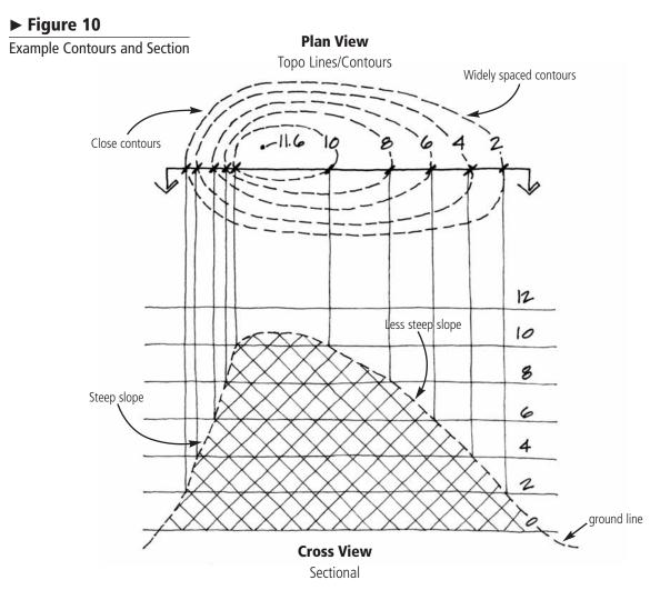
Contour lines represent each step in elevation of the ground at a specific contour interval (e.g. each one, two or five foot increase in elevation might be marked). Steep slopes result in close contour lines while widely spaced contour lines result from the plotting of gentle grade changes.
