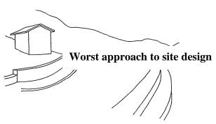
This example illustrates the use of unnecessary retaining walls and terraces. Massive modifications to slopes such as this are often highly visible and are not recommended.
