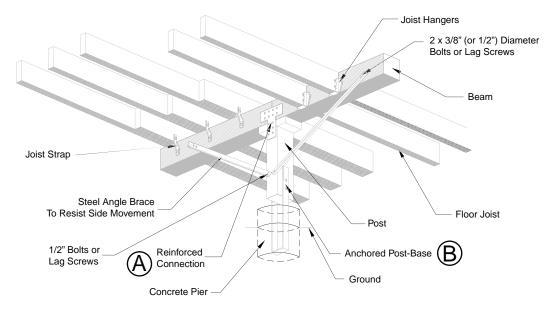
Figure 18: Post-and-Pier Foundation
