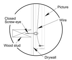
wall studs. Use a stud finder to find the most secure location to attach them to the wall.
