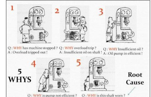
A : Pump drive shaft worn !
