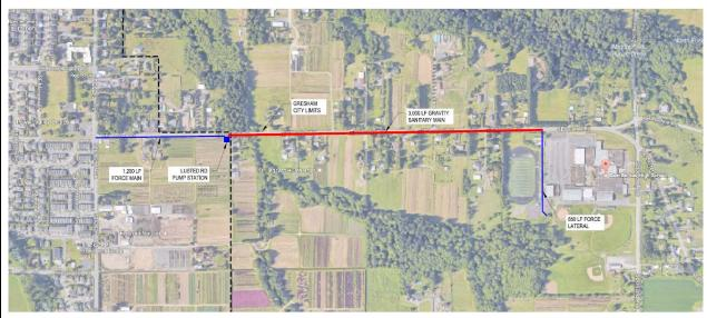
Figure 3. Proposed sewer pipe alignment
