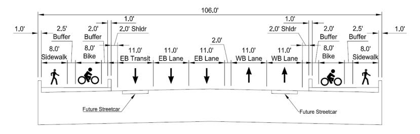
ALT3 - Main Span Bridge Typical Section (Looking West)
