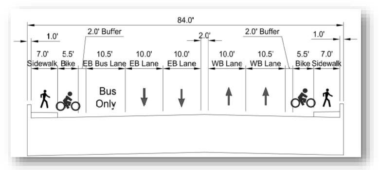
Main Span Bridge Typical Section (Looking West)
