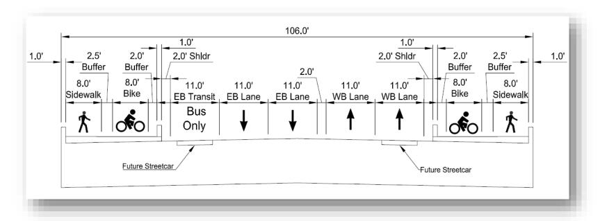
Main Span Bridge Typical Section (Looking West)
