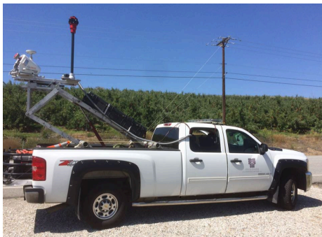
The LiDAR truck used to capture the data for this project.
