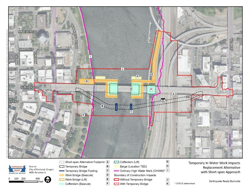
Figure 3.17-4 Temporary In-Water Impacts – Short-Span Alternative
