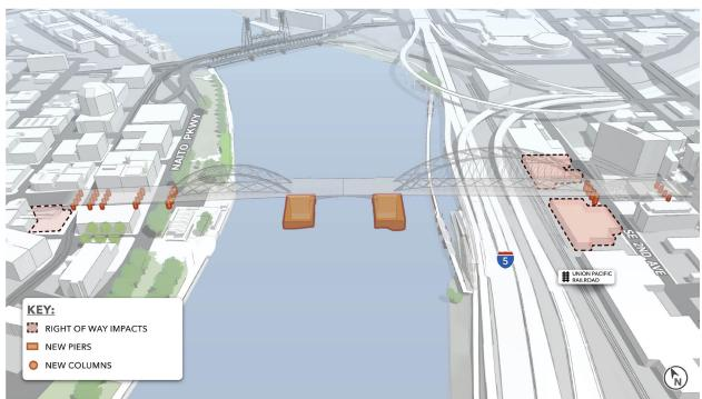
Figure 9. Long-Span Alternative: Configurations and Bent Locations (Tied-Arch Configuration with Generic Movable Span Shown)
