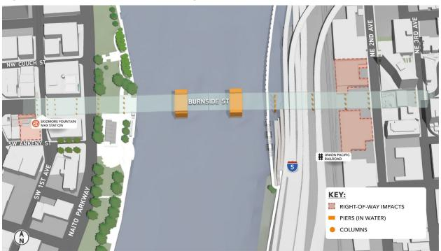
Figure 5. Short-Span Alternative: Configurations and Bent Locations
