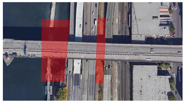
**Concept #2** - Ground improvements are proposed at Bents 9 through 12 as shown in Figure 12. It is anticipated that the ground improvements extend down to the Troutdale Formation subsurface layer. Additionally, the improvement sites have been sized to increase stability and withstand the large-scale soil displacements that will occur during a seismic event at each bent.
