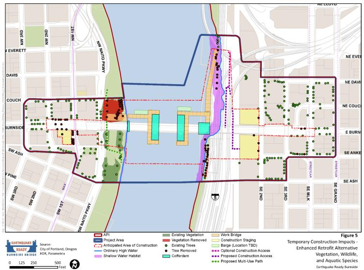
Figure 5. Temporary Construction Impacts (Retrofit Alternative)
